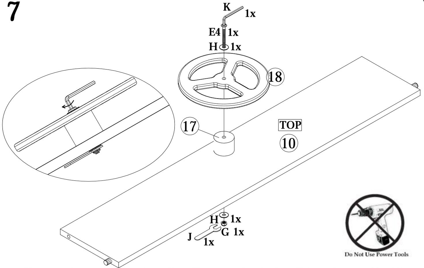
Using the Spanner (J) and Allen Key (K), ensure that the Bolt (E4) and Locking Nut (G) are securely fixed and that the wheel can still turn freely.
