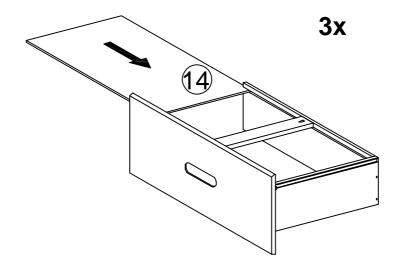
Step 7 DO NOT use any power tools as this may damage the frame and will invalidate any claim.
